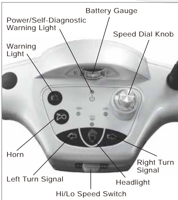
Figure 2 - HS-890 Control Panel
