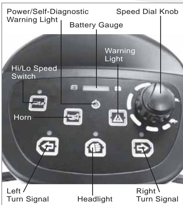
Figure 2 - HS-898 Control Panel
